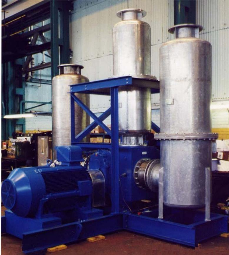
Chiltern Acoustics Ltd reactive silencers fitted to a Dresser 1431 DVJ exhauster
