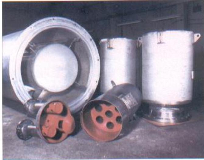
A selection of gas vent silencers showing the smaller range silencers. The unit at the bottom photographed before final assembly shows multiple inlets where a single silencer is being used to reduce noise from different valves. The absorption section for this unit is a 7 seven tube section.
