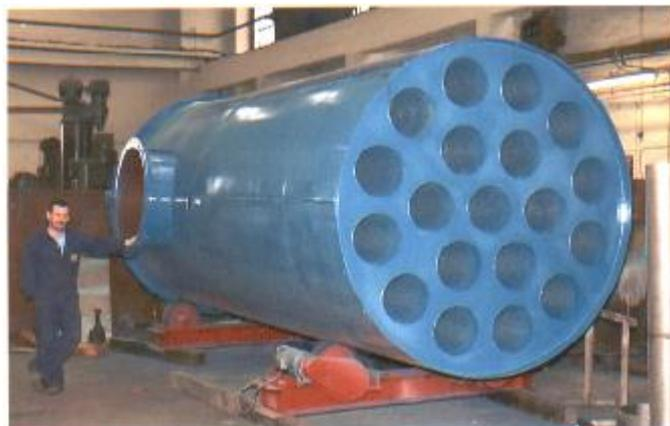
A larger vent silencer design to stand vertically on the ground with a side inlet- 19 tube absorption section.
