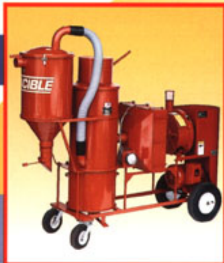
Model 4594 equipped with HEPA filter, magnetic gauge, pneumatic tires, manual bag shaker, integral auxiliary collector mounted on a common base, and automatic gravity dump discharge valve. Equipment used to recover tungsten carbide from pits.
