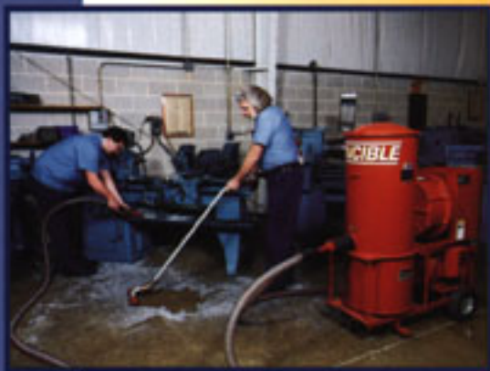
Machining center runs two operators for cleaning floors and machinery areas. Valuable resalable metals are reclaimed. A safer, more productive work environment is in place as brooms and air nozzles are replaced by a vacuum system.
