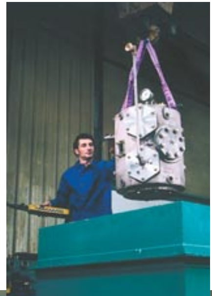
Helium leaktest and Hydrostatic Test (soap bubble, mass spectrometer)
