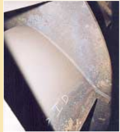
Impeller being prepared for blade tail extensions to increase performance
